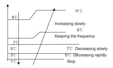
The compressor stops for more than 3 minutes, Tpg\_indoor>  $9^{\circ}$ C, the compressor recovers.
