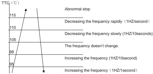
TTC>=115°C lasts for 20 seconds. Overheating protection of air-blowing, alarm malfunction to the indoor, others don't last.
