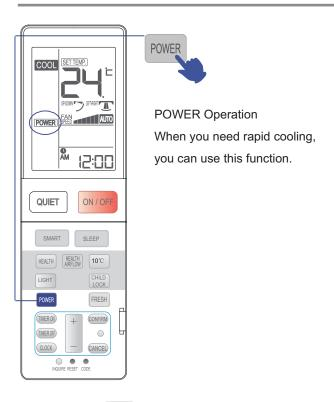
For each press, **POWER** is displayed Air conditioner starts POWER function operation.
