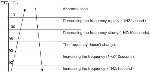
TTC>=110°C lasts for 20 seconds. Overheating protection of air-blowing, alarm malfunction to the indoor, others don't last.
