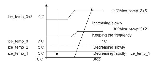
When Tpg\_indoor  $\langle$  ice\_temp\_1°C, the frequency of the compressor decreases at the speed of 1HZ/1second.
